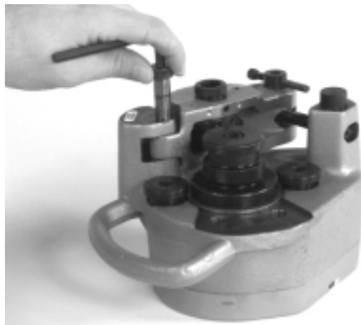
Figure 14 – Removing Shoulder Screw
