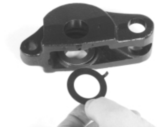
Figure 18 – Inserting Tabbed Thrust Washer
